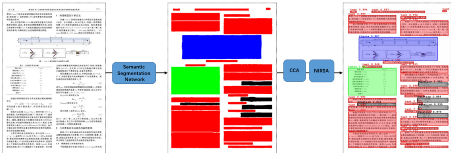
Fig. 1. Illustration of our method. The results of both pixel-wise and region-wise segmentation are shown in the rightmost image, where each region is represented by a bounding box, corresponding label and confidence score (white: background, red: text, green: table, blue: figure, black: formula) (Color figure online).
